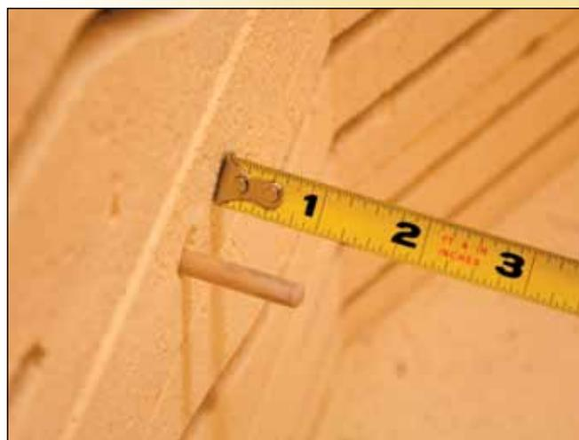
*As a rule of thumb, the thermocouple should extend into the firing chamber by four times its diameter. Bumping the thermocouple with a shelf and pushing it into the wall of the kiln will cause the kiln to get too hot.*
