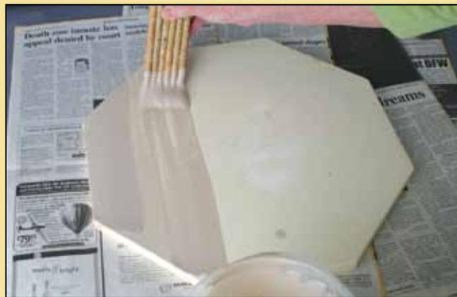
*Start the brush stroke an inch or so from the edge of the shelf and work toward the opposite side. This avoids buildup of kiln wash on the edges.*
