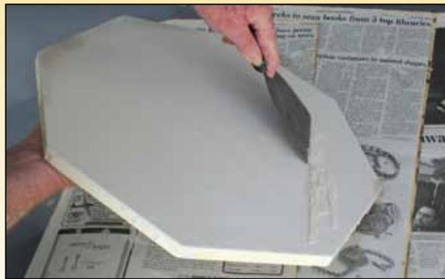
*If glass sticks to the shelf, scrape it off with a putty knife at a sharp angle. Wear safety glasses, since sometimes chipped glass becomes airborne.*
