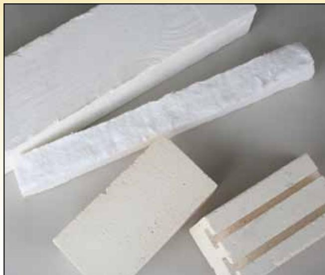
*Kilns are insulated with either ceramic fiber or insulating firebricks. Ceramic fiber heats and cools more rapidly than firebricks, while a firebrick kiln is more suitable for long annealing times.*
