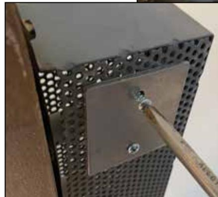
*In this photo, a shim was added that pressed the lid switch down so that the elements would stay on while the kiln fired.*
